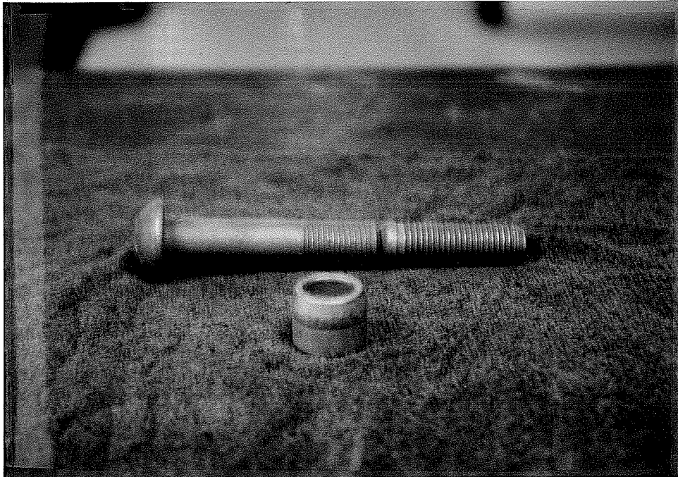
Figure 2.2: Huck C50L fastener and LC collar
